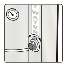
Turn the thermostat knob to the desired setting. The indicator light comes on when the heating element is heating the water.
